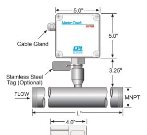
Two-wire, twisted pair interconnect cable required between Remote Electronics and Flow Transmitter (max. 5 ohm resistance).
